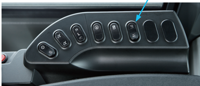
Remote positioner switch Boom / Bucket
